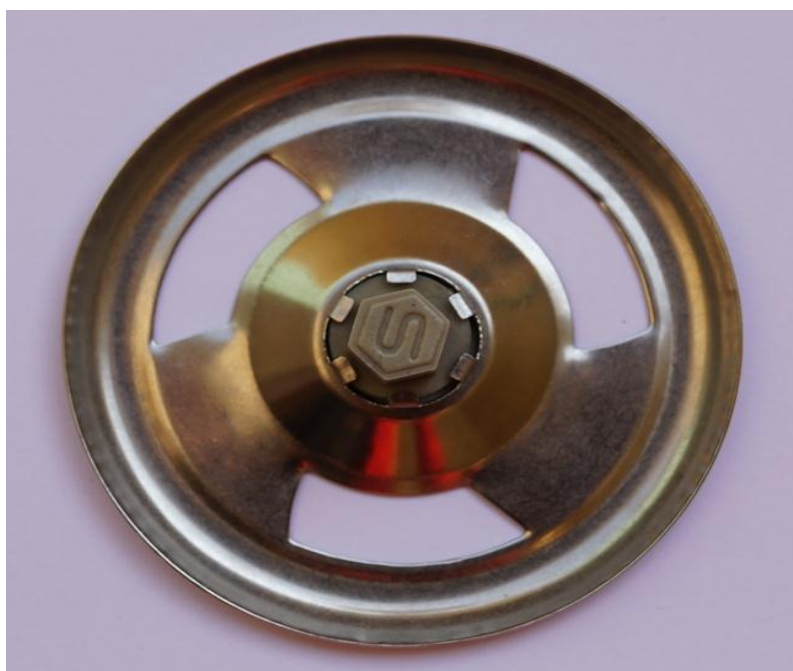
Fig. 1: Disc type blade used to dehull the sunflower seeds (Top view)
