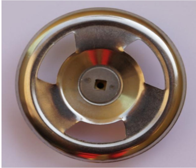
Fig. 2: Disc type blade used to dehull the sunflower seeds (Bottom view)
